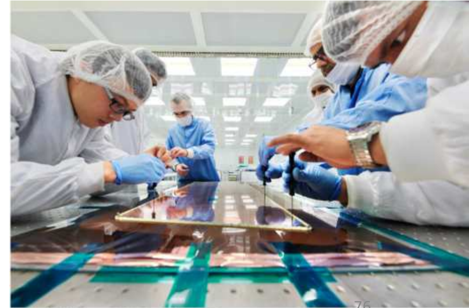
Assembly of the GEM detectors at CERN in clean room (Image: CERN)
