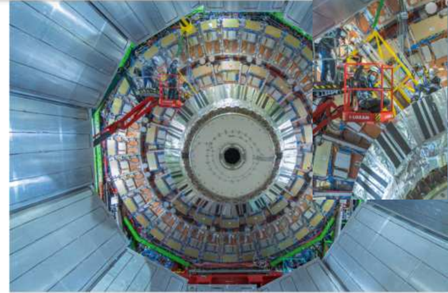
The last installation of Gas Electron Multiplier (GEM) detectors on the second CMS endcap took place in September. (Image: CERN)
